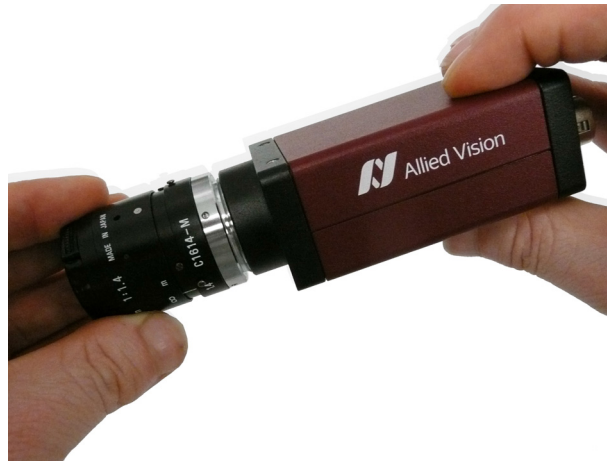
Figure 118: Illustration of camera orientation when removing lens or dust cap
