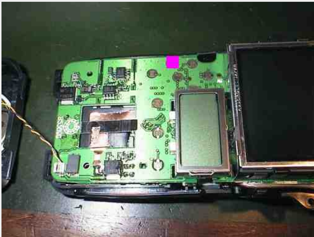
Fig. 2 Remove the speaker leads and the screw marked
