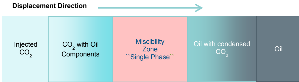
Figure 4: Illustration of the zones that develop in miscible CO 2 flooding.
