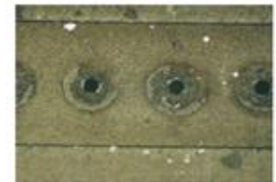
Used head, nozzles open but corrosion → Jet angle problems
