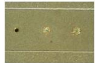
Used head, 1 nozzle open, 2 nozzles clogged
