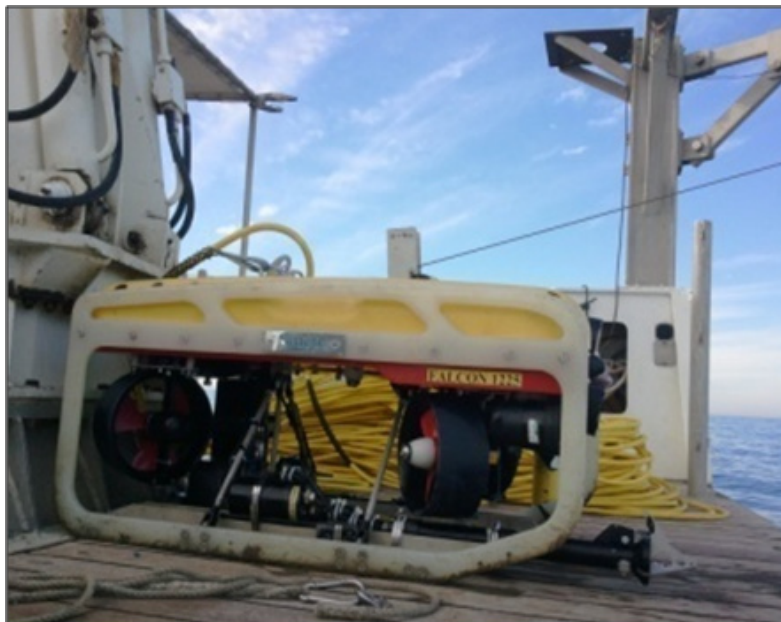
Image 1. Seaeye Falcon ROV used during the Post-Drill survey.
