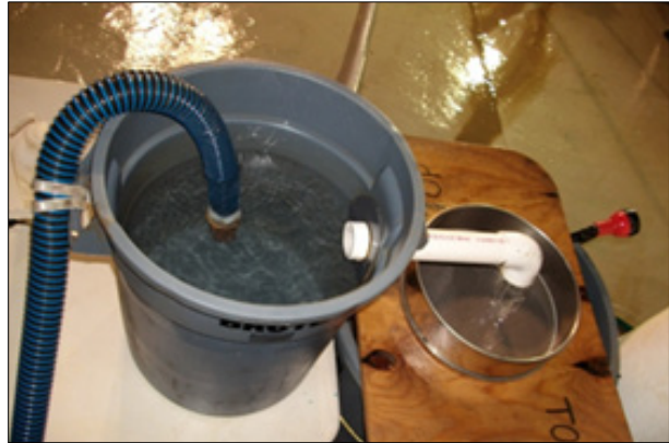
Image 4. Macrobenthic infaunal sieving apparatus consisting of an upper mixing barrel and sieve table over a lower spillover barrel.
