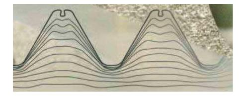
Representation of a roll formed internal thread.
