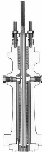
Figure 1-6. Bellows Seal Bonnet
