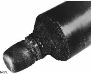
Figure 5-7. Typical Appearance of Cavitation Damage
