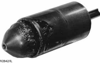
Figure 5-6. Typical Appearance of Flashing Damage
