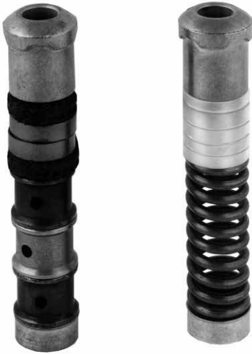
Figure 8-5. Typical Valve Stem Packing Assemblies
