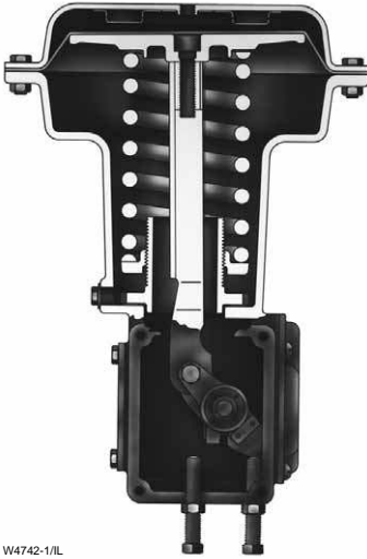
Figure 3-34. Diaphragm Actuator for Rotary Shaft Valves
