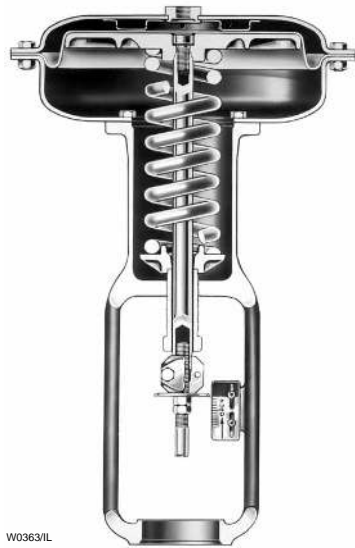
Figure 8-4. Typical Spring-and-Diaphragm Actuator
