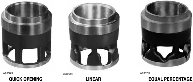
Figure 3-28. Characterized Cages for Globe-Style Valve Bodies
