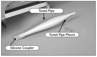
• 4. Carefully remove the tuned pipe by sliding the silicone coupler apart from the exhaust header.
