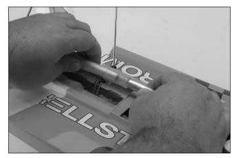
O 8. Re-attach the tuned pipe and coupler to the exhaust manifold.
