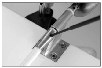
O 6. Carefully re-install the flex shaft and nylon bushing, making certain that you correctly tighten the collet nut. Next, re-install the drive shaft and propeller and tighten setscrews on the flats of the drive shaft.
