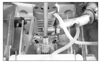
O 3. Turn on your radio system and attach a fully charged glow igniter (DYN1925) to the glow plug. Insert the starting wand into the Tiger Drive and actuate the starting switch until the engine begins to run. If the engine does not start, place your index finger over the carburetor and actuate the starter until you see fuel enter the carburetor through the fuel line.
