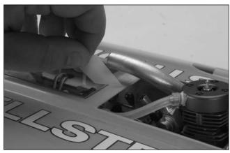
O 7. Re-install the battery holder back into the radio box and properly seal the radio box with clear tape. Failure to properly seal the radio box could result in damage to your radio equipment.
