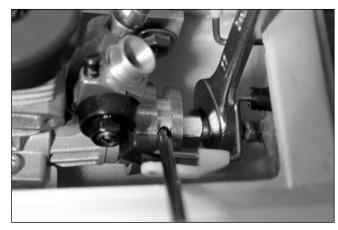
3. Insert a hex driver into the hole located on the flywheel to lock the crankshaft in place. Then use an 10mm wrench to loosen the collet nut.
