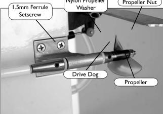
O I. Carefully note how the drive shaft and prop are presently installed. This is important so that when you have finished lubricating the drive shaft, you can correctly re-install the drive shaft.
