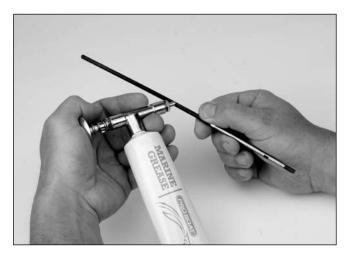
O 5. Liberally lubricate the entire length of the flex shaft with silicone cable grease as shown.
