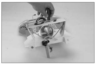
O 3. Use a 2.5mm Allen wrench to remove the tuned pipe mount as shown above.
