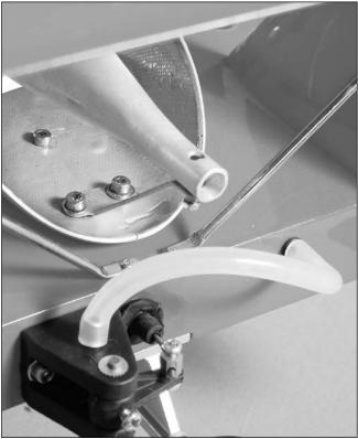
O 9. Re-install the tuned pipe mount.
