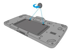
2. Remove the back cover and pull the battery out.
