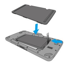
3. Lock the two screws on the battery cover by turning clockwise.
