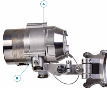
Figure 2-6: Closing Security Screw
