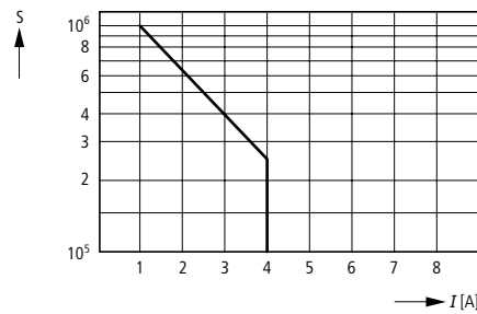
Contact life Operations S 220 V 50 Hz AC-1 360 operations/h
