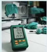
**SD700** Barometric Pressure/ Humidity/Temperature Datalogger (p. 83)
