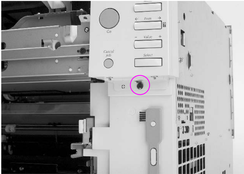
Figure 6-11 Control panel removal and replacement
