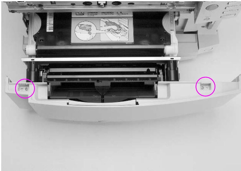
Figure 6-9 ITB drawer (middle drawer) cover removal and replacement
