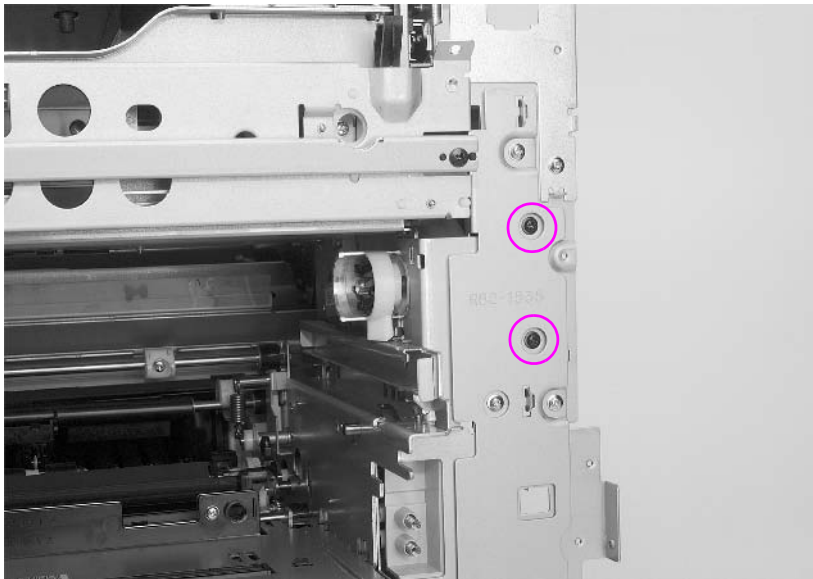
Figure 6-36 Drum drive assembly removal and replacement (3 of 3)
