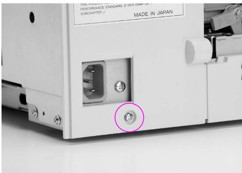
Figure 6-6 Right rear cover removal and replacement
