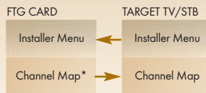
figure 2. DATA FLOW-BETWEEN FTG CARD AND TARGET TV/STB Conditions of HCS1410: Previously used in a TV/STB of the same model.
