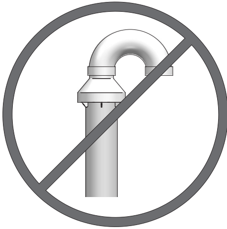
Figure 5-5 Do Not Install U-Bend to Rain Cap
