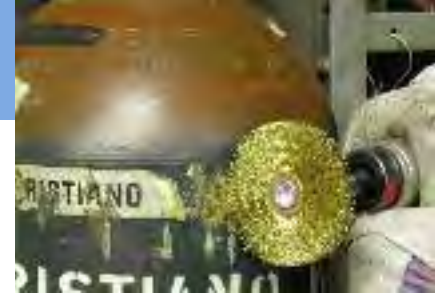
Removing labels from a compressed-gas storage cylinder.
