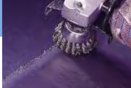
Removing slag from a flame-cut steel plate.
