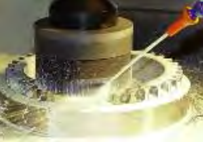
Deburring a bearing cage in a CNC machining center.
