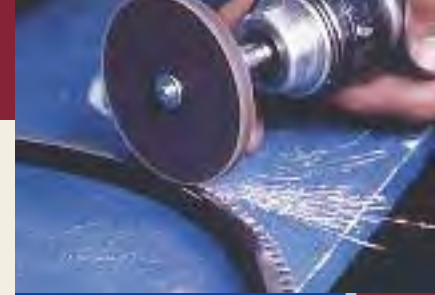
A unitized wheel deburring a ring gear.
