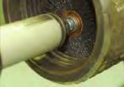
Cleaning internal threads inside a valve.
