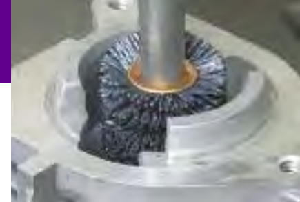
Deburring the internal bores of an air-cooled cylinder head.
