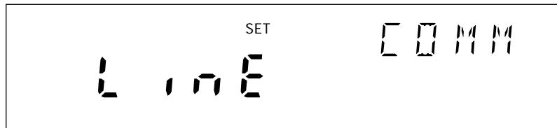
Communications display for setting the line frequency
