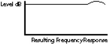
PCC receiving direct sound and reflected sound nearly simultaneously.
