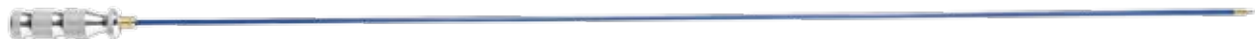
Cleaning Rod , steel with plastic coating, with ball bearing mounted aluminum handle 33650-10 5 mm, 100 cm long PU 5 33650-11 6 mm, 100 cm long PU 5
