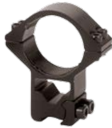
Scope Mount 2-part light metal slide-on mount with double screwing for 11 mm dovetail, 30 mm Ø, height 25 mm 37308-06
