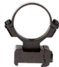
Brno Scope mounts Steel, 2-part slide-on mount for rifles with 19,5 mm dovetail (Brno Mod. ZKK 600, 601, 602, 537) 37307-01 1" Ø, height 17 mm 37307-03 30 mm Ø, height 17 mm 37307-02 1" Ø, height 22 mm 37307-04 30 mm Ø, height 22 mm
