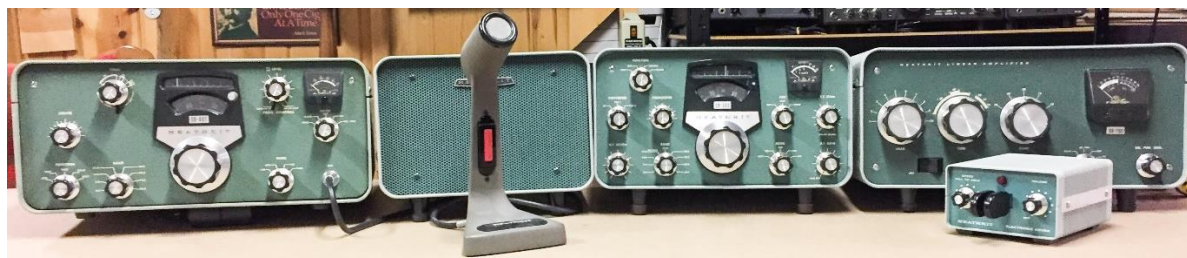
The W9MXQ Heathkit Twins Station with their Linear Amplifier SB-401 Transmitter, SB-600 Speaker, SB-303 Receiver, SB-200 Amplifier W9MXQ Collection
