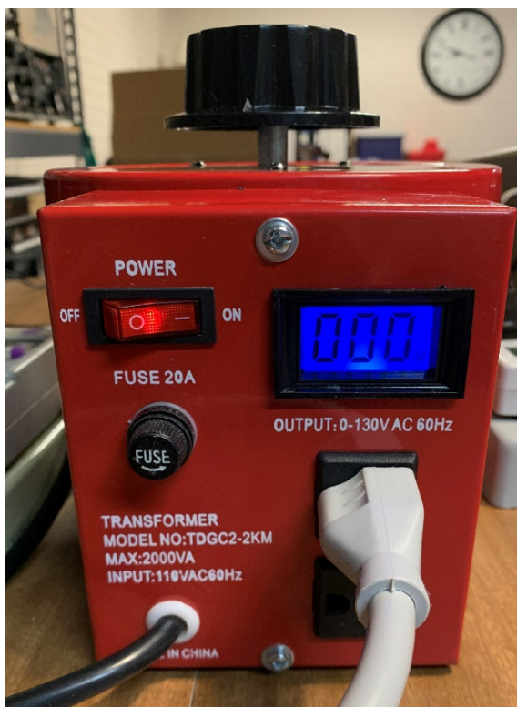
Autotransformer powered on and voltage set at Zero Volts
