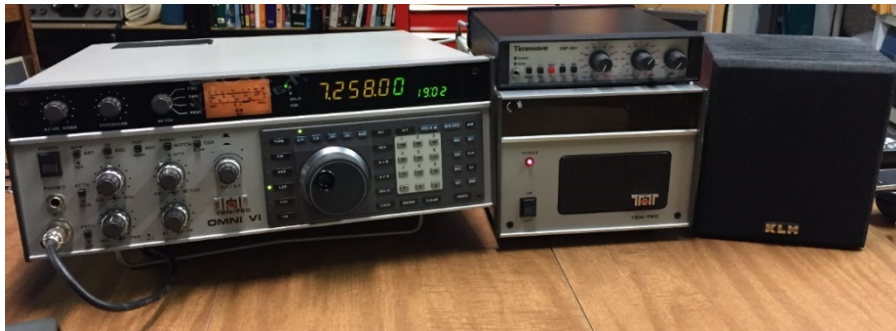
Left to Right Omni VI HF Transceiver & 962 AC Power Supply Shown with Timewave DSP-59+ Audio DSP Unit & KLH Bookshelf Speaker W9MXQ
