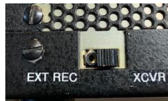
The troublesome Switch can be locked in one desired position by inserting a #4-40 hex nut, as shown. The nut can be held in place with tape (not shown here).
