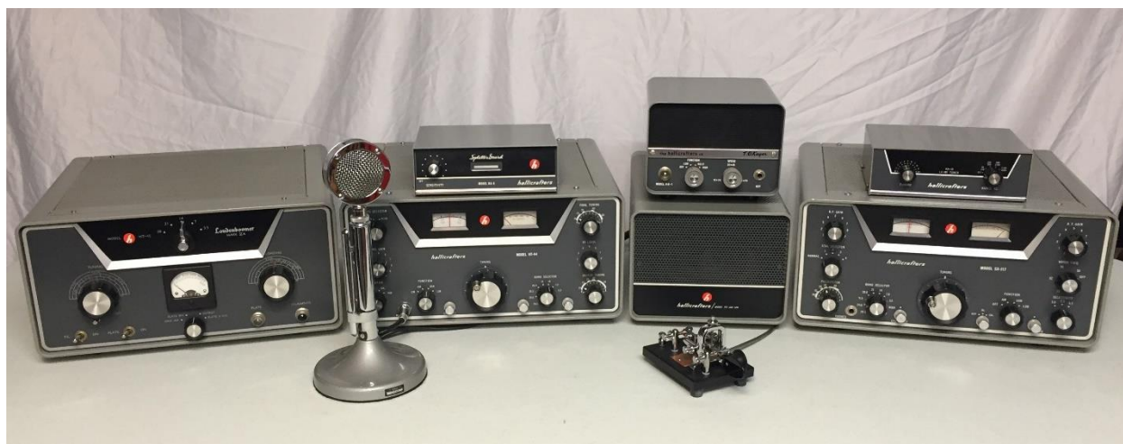
The W9MXQ Hallicrafters Twins Station with their Linear Amplifier HT-45 Amplifier, HT-44 Transmitter, PS-150-120 Console, SX-117 Receiver W9MXQ Collection
