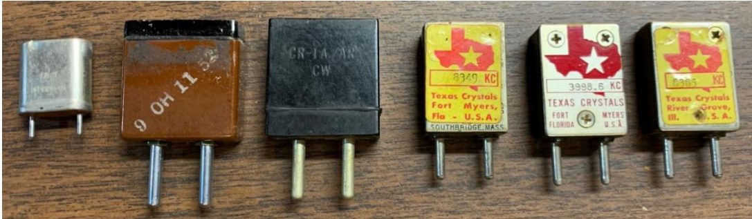
Typical Crystals used by Novice (and other) Class Licensees (Note that these are not necessarily ham radio band crystals!)
