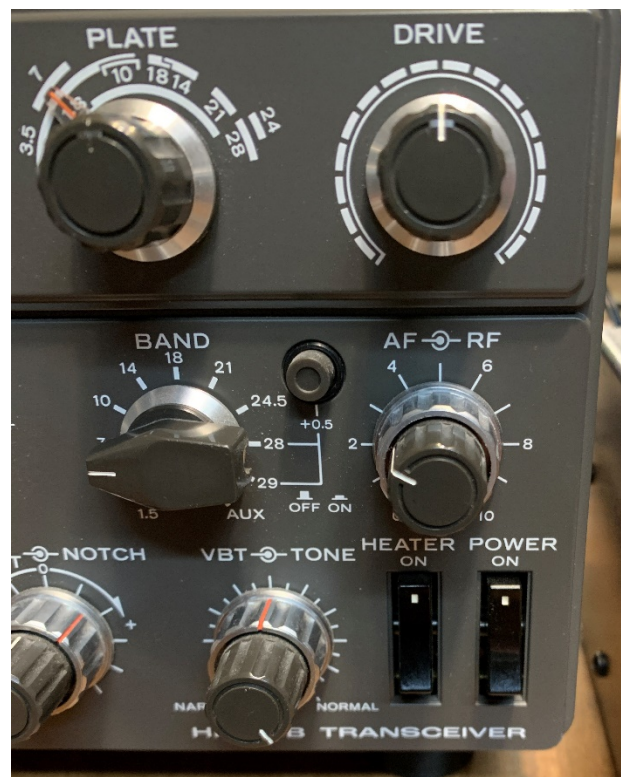
Radio shows both power switches “ON” and AF Gain at about 30% level
