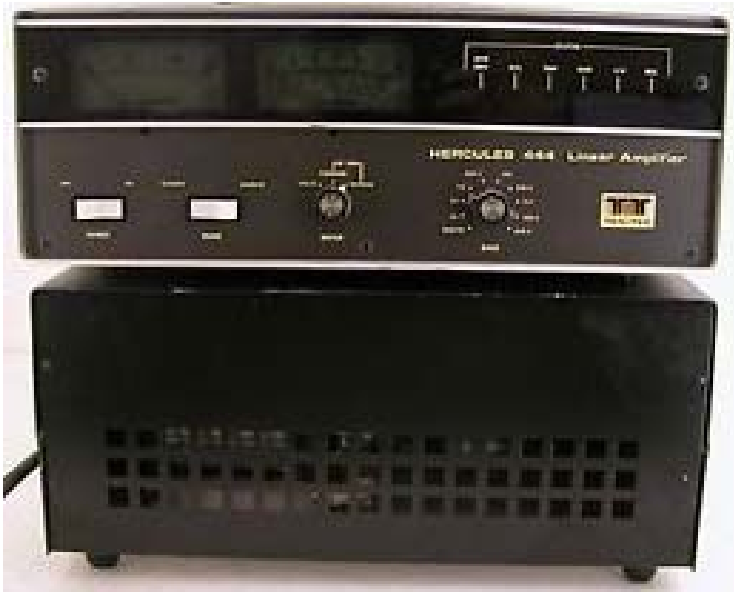
Ten-Tec Model 444 Hercules Linear Amplifier (sitting on top of matching AC Power Supply)
