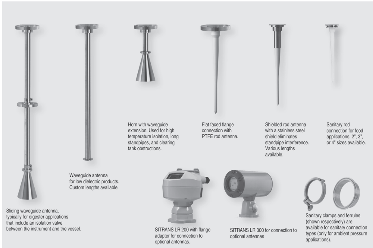
Antenna configurations for SITRANS LR200 and LR300
