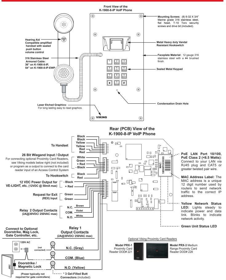
Note: The gel-filled (water-tight) butt connectors are designed for insulation displacement on 19-26 gauge wire with a maximum insulation of 0.082 inches.
