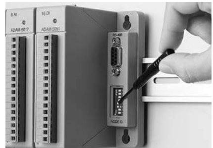
Node ID Setting 8-pin dip switch configuration
