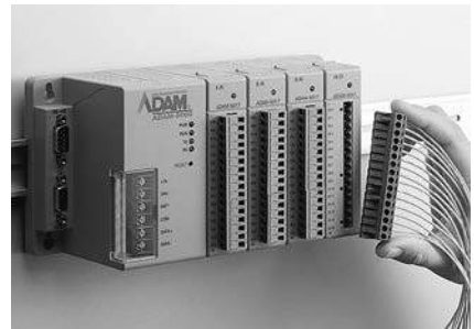
Connection Pre-wired plug-in terminals with I/O modules
