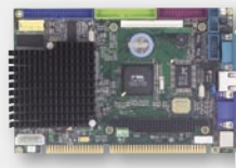
Vega86-6242 Half-size ISA Bus SBC 7.24 x 4.80 inches (184x122mm)
