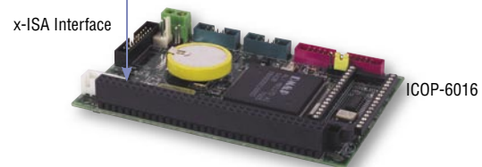
VGA function support via x-ISA interface
