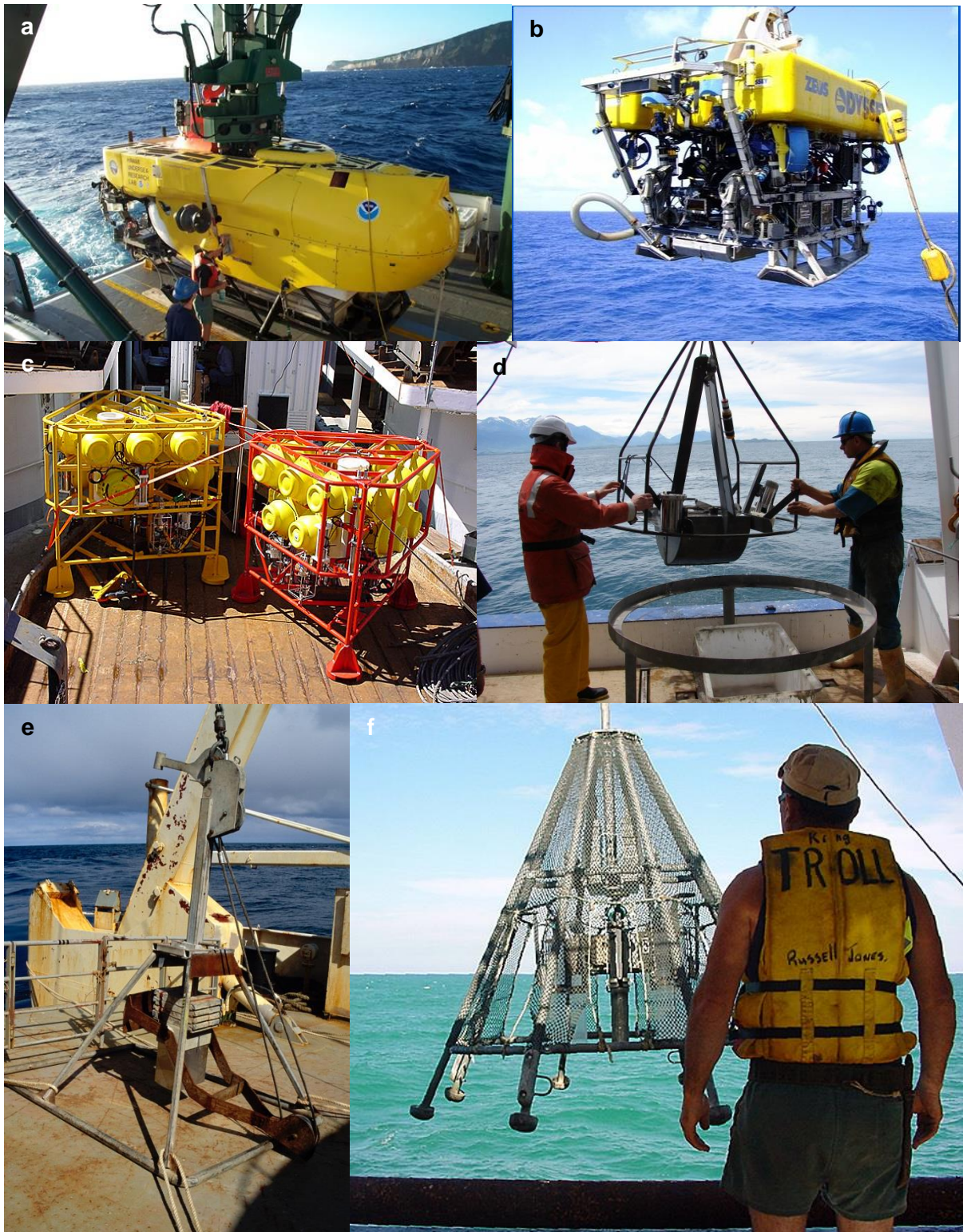
Figure 6-1: Point sampling of the seabed. (a) Pices crewed submersible, (b) Odyssey remotely operated vehicle, (c) benthic lander, (d) van Veen grab in closed position, (e) Reineck box corer, (f) multicorer (all images NIWA).
