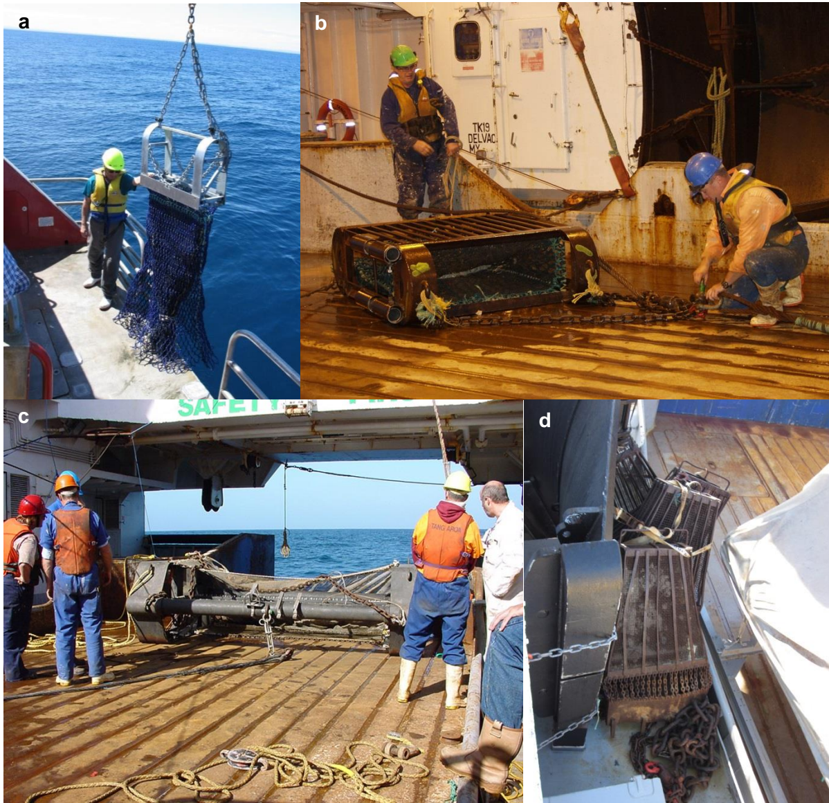
Figure 6-3: Mobile sampling of the seabed. (a) small epibenthic sled, (b) large epibenthic sled, (c) Agassiz beam trawl, (d) rock dredge and spares on RV Tangaroa (all images NIWA).
