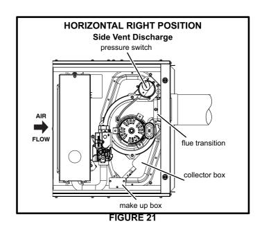
The SL280UHV series units are classified as fan-assisted Category I furnaces when vertically vented according to the latest edition of National Fuel Gas Code (NFPA 54 / ANSI Z223.1) in the USA. A fan-assisted Category I furnace is an appliance equipped with an integral mechanical means to either draw or force combustion products through the combustion chamber and/or heat exchanger. The SL280UHV is not approved for use with horizontal venting..
