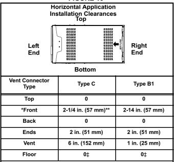
\*Front clearance in alcove installation must be 24 in. (610 mm). Maintain a minimum of 24 in. (610 mm) for front service access. \*\* 3-1/4 in. if single wall vent pipe is used.
