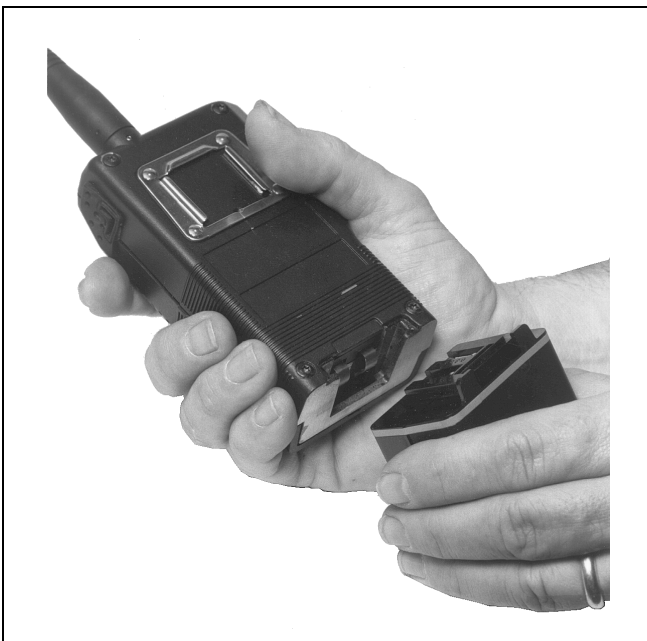
Figure 5 - Removing The Battery Pack
