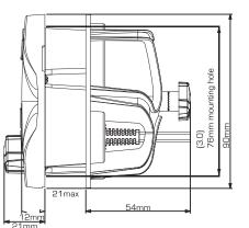
**Note:** The remote should be mounted on no more than a 45° angle from the verticle plane.
