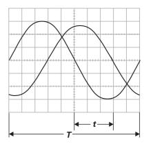
In the example illustrated, t = 3div. and T = 10div. The phase difference in degrees is calculated from
