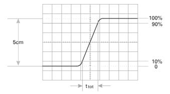
With a time coefficient of  $0.05\mu$ s/div. and X x10 magnification, the example shown in the above figure results in a total measured risetime of
