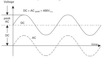
The dotted line shows a voltage alternating at zero volt level. If superimposed on a DC voltage, the addition of the positive peak and the DC voltage results in the max. voltage (DC + ACpeak).
