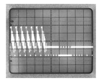
MODE: DEL (DELAY) TIME/DIV: 0.1ms/div Trigger coupling: TV-F Trigger slope: falling ( - ) Delay time: 20ms
