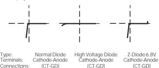
The polarity of an unknown diode can be identified by comparison with a known diode.
