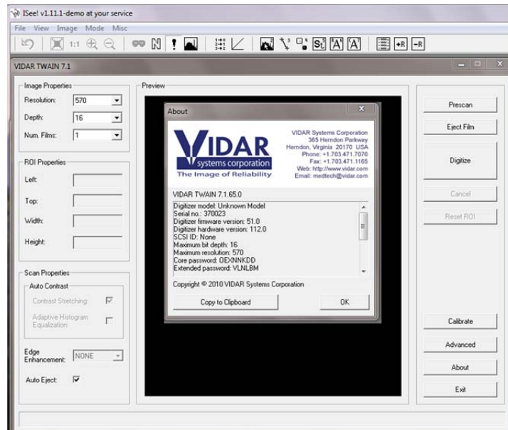
Fig.1: The TWAIN interface used for image acquisition from the scanner "Vidar NDT Pro".
