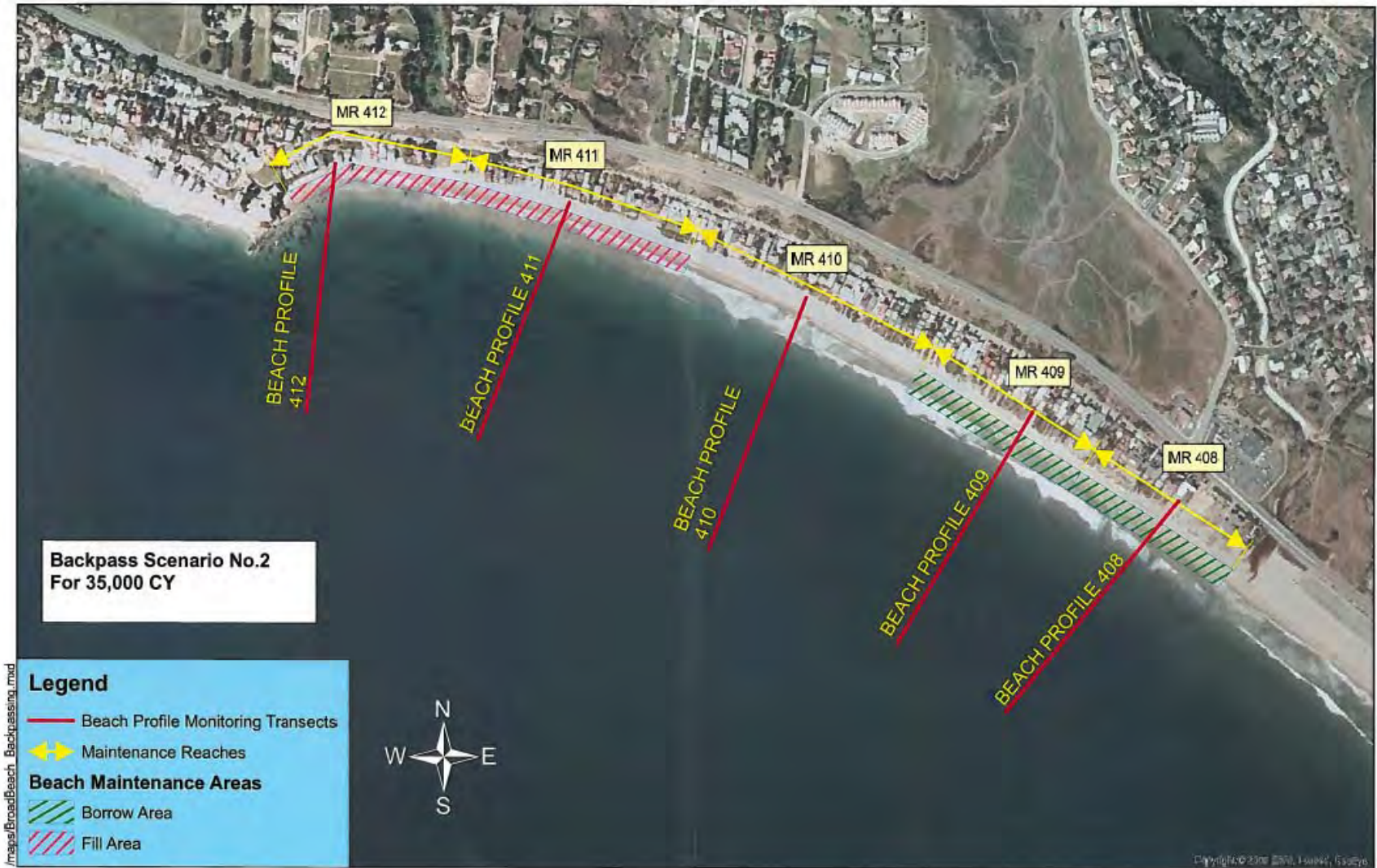
Figure 12. Proposed Backpass Scenario 2 for Removal of 35,000 cy from Combined MR 408 and MR 409 at East for Placement at MR 411 and MR 412 in West End
