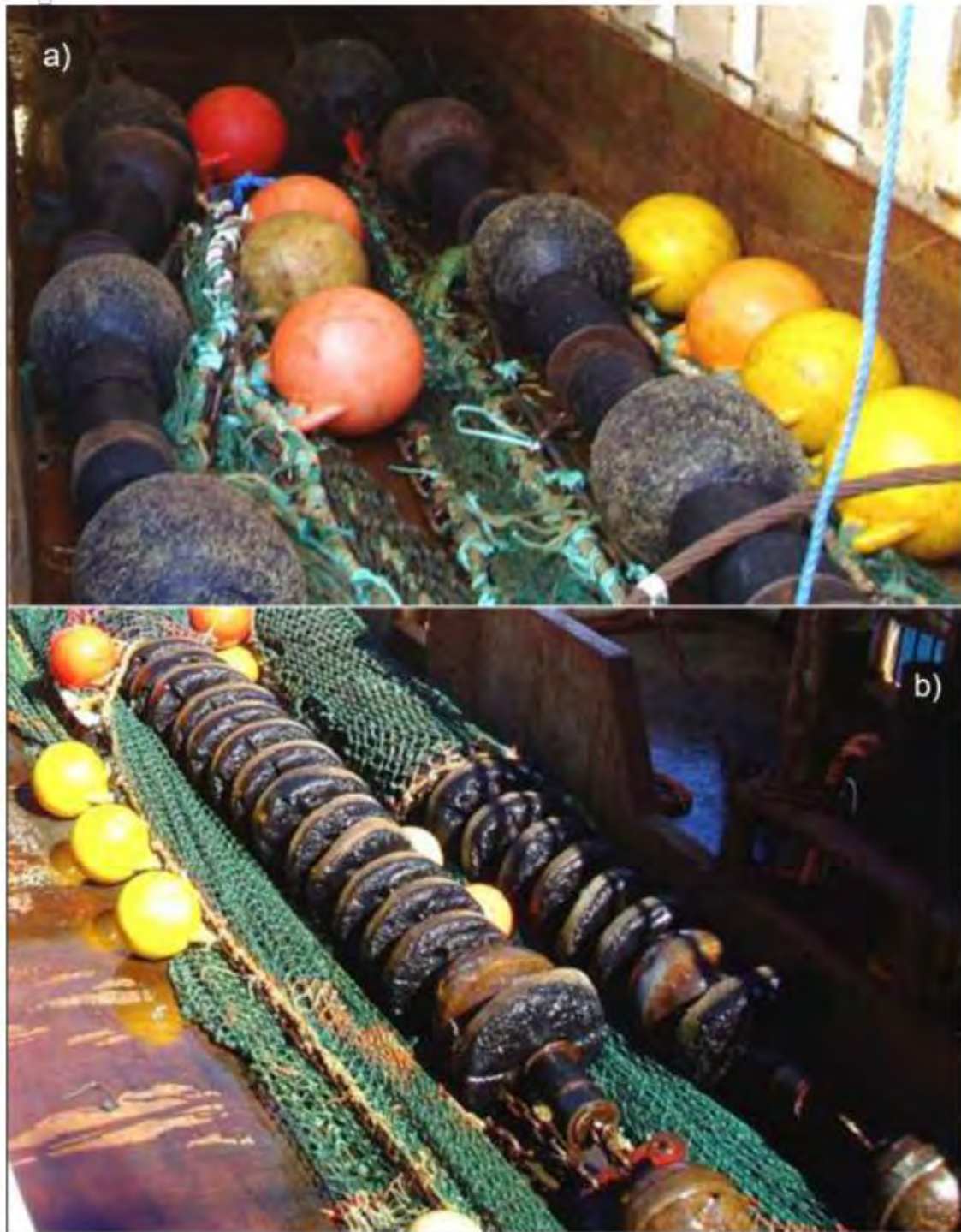
Figure 5: Typical ground-gear configurations used by New Zealand-flagged vessels when bottom trawling for orange roughy and oreos showing ground-ropes equipped with a) 50–60 cm rubber bobbins separated by rubber spacers, and b) with more closely spaced 60–80 cm ‘rockhopper’ rubber discs plus leading end steel bobbins.
