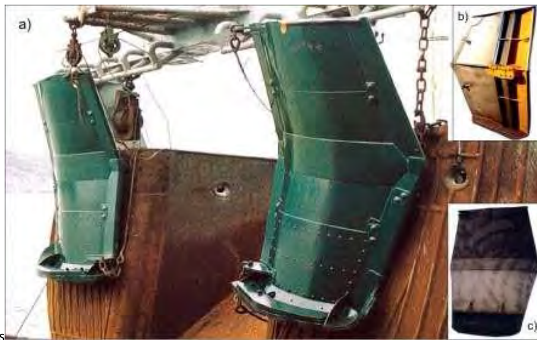
Figure 4: Examples of trawl doors in use on New Zealand-flagged vessels using bottom trawls for orange roughy and midwater trawls for benthopelagic species like alfonsinos. a) Nichimo Super-Vee doors rigged on a trawler stern, b) a Morgere WX door and c) a Morgere WV door.
