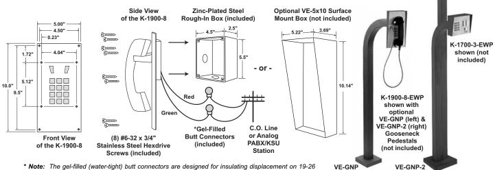
\* Note: The gel-filled (water-tight) butt connectors are designed for insulating displacement on 19-26 gauge wire with a maximum insulation of 0.082 inches. Cut off stripped wire ends before terminating.
