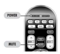
**IMPORTANT:** You have 30 seconds to perform the next step while you are in programming mode. If you do not press a button within 30 seconds, the component LED light will turn off. The remote will exit the programming mode and you will have to start over.
