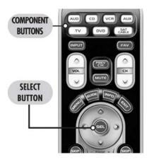
**IMPORTANT:** You have 30 seconds to perform the next step while you are in programming mode. If you do not press a button within 30 seconds, the component LED light will turn off. The remote will exit the programming mode and you will have to start over.
