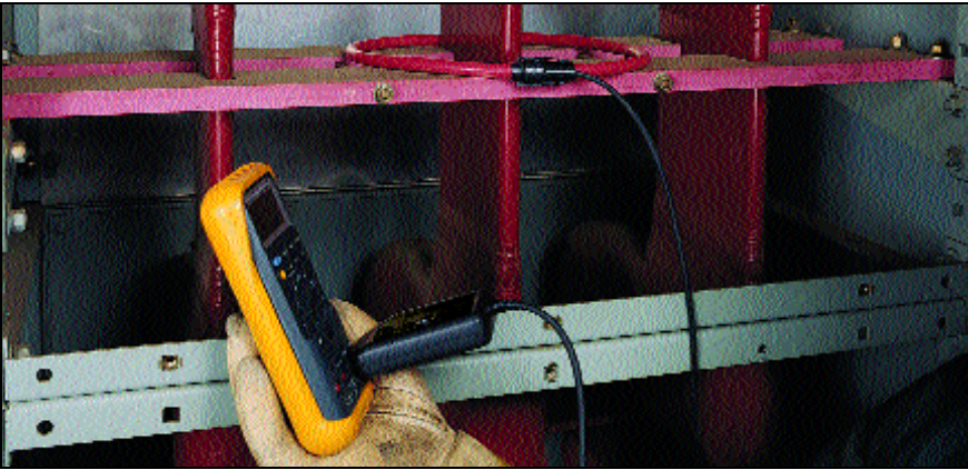
Direct connections to DMMs, or use BNC accessory to connect to oscilloscopes
