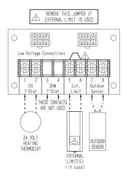
Figure 11.3: Low Voltage PCB Terminal Connections
