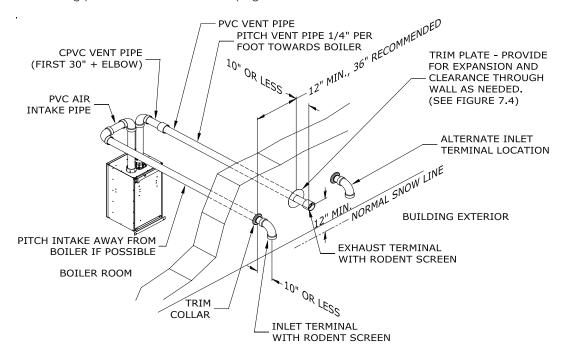
Figure 7.6: Horizontal CPVC/PVC Venting, (Vent Option #1, Terminal Option A)
