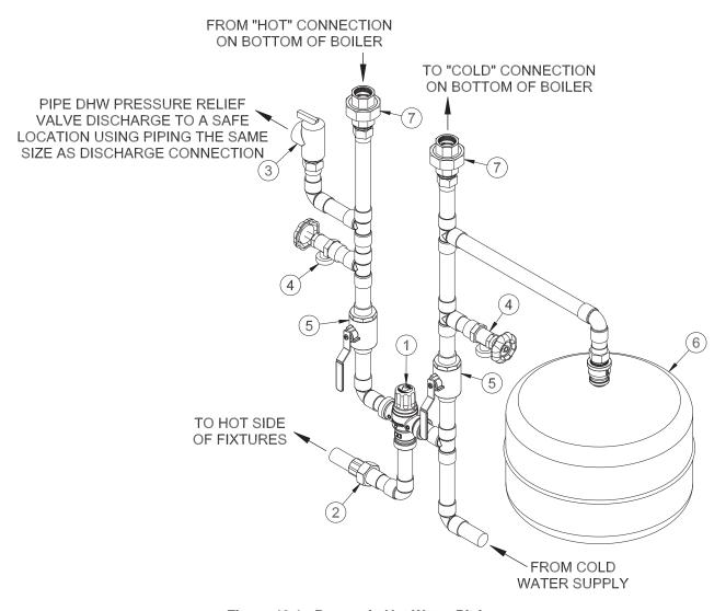
Figure 10.1: Domestic Hot Water Piping
