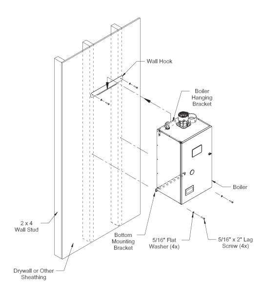
Figure 5.2 Boiler Mounting Bracket Installation / Boiler Wall Mounting
