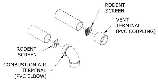
Figure 7.28: Installation of Standard Horizontal Terminals
