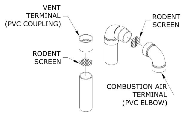
Figure 7.29: Installation of Standard Vertical Terminals
