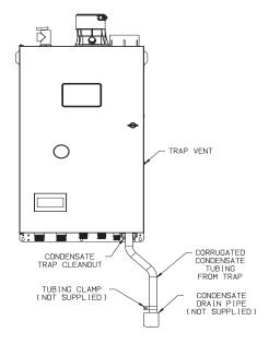
Figure 7.47: Condensate Piping Arrangement
