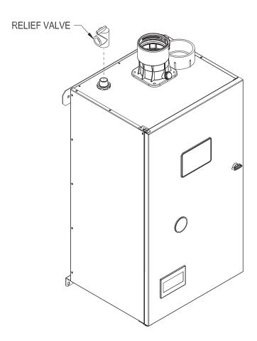
Figure 9.0: Factory Supplied Piping and Trim Installation
