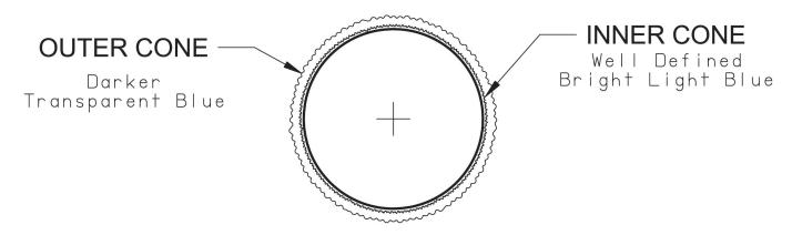
Figure 12.3: Burner Flame
