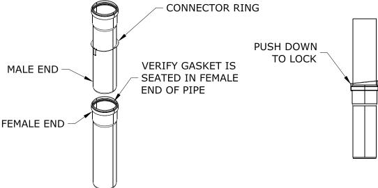
Figure 7.44: InnoFlue Connector Ring Installation
