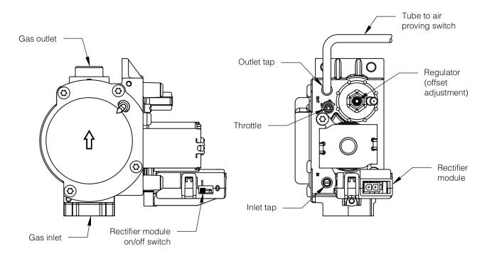
Figure 12.4: Gas Valve Detail
