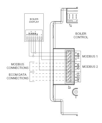
Figure 11.6: J3 Field Wiring
