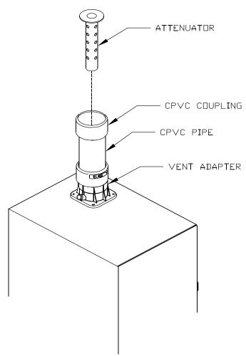
Figure 7.1A: Installation of Vent Side Attenuator
