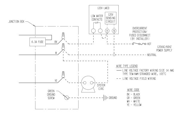
Figure 11.4a: 120 Volt LWCO Field Wiring
