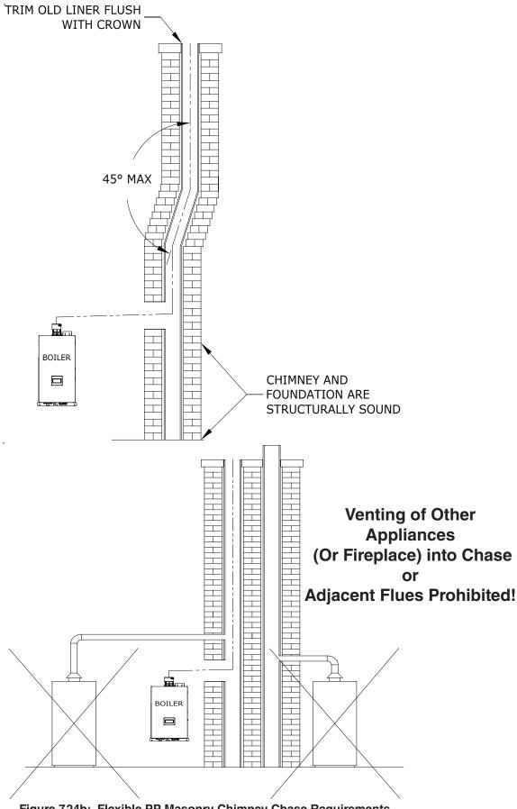
Figure 7.24b: Flexible PP Masonry Chimney Chase Requirements
