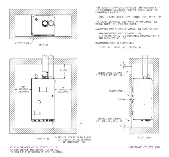
Figure 4.1: Minimum Clearances To Combustible Construction
