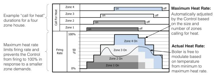
Figure 13.11: Four Zone House (with Sage Zone Control Connected)
