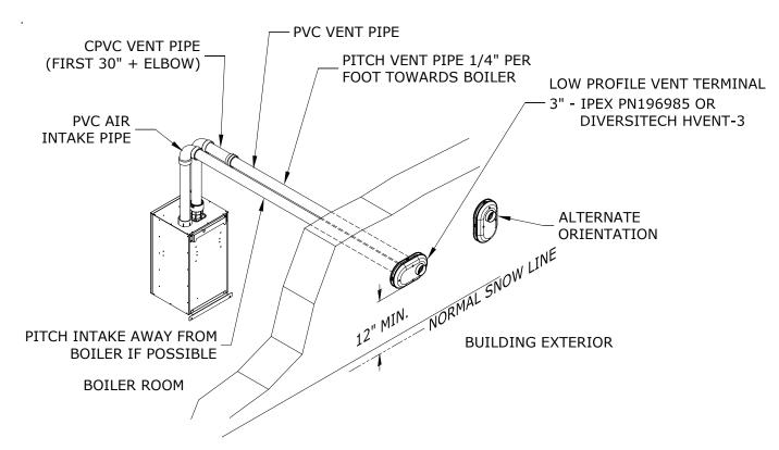
Figure 7.7: Horizontal CPVC/PVC Venting with Low Profile Terminal, (Vent Option #1, Terminal Options B & C)
