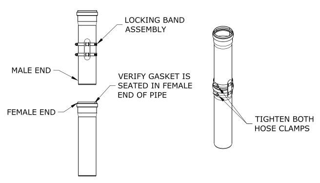
Figure 7.41: Polyflue Pipe Locking Band Installation
