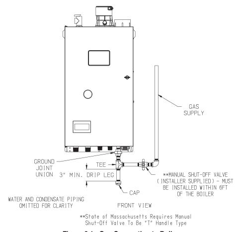
Figure 8.1: Gas Connection to Boiler
