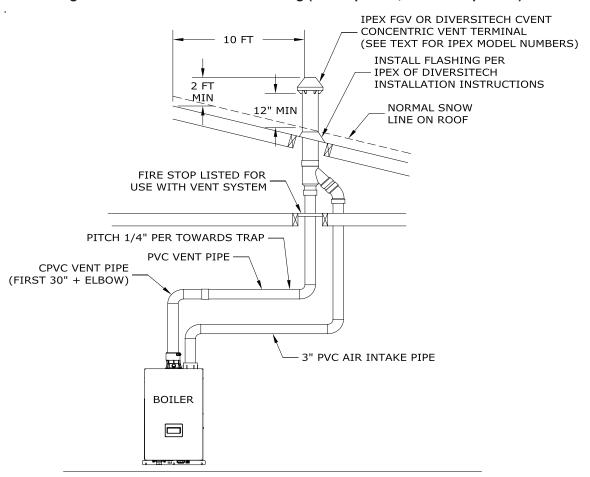
Figure 7.16: Vertical CPVC/PVC Venting with IPEX Concentric Vent Terminal (Vent Option 5, Terminal Option I, J)
