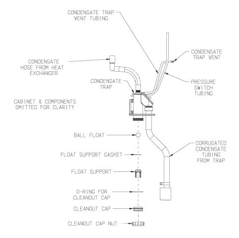
Figure 14.3: Condensate Trap Exploded Parts View
