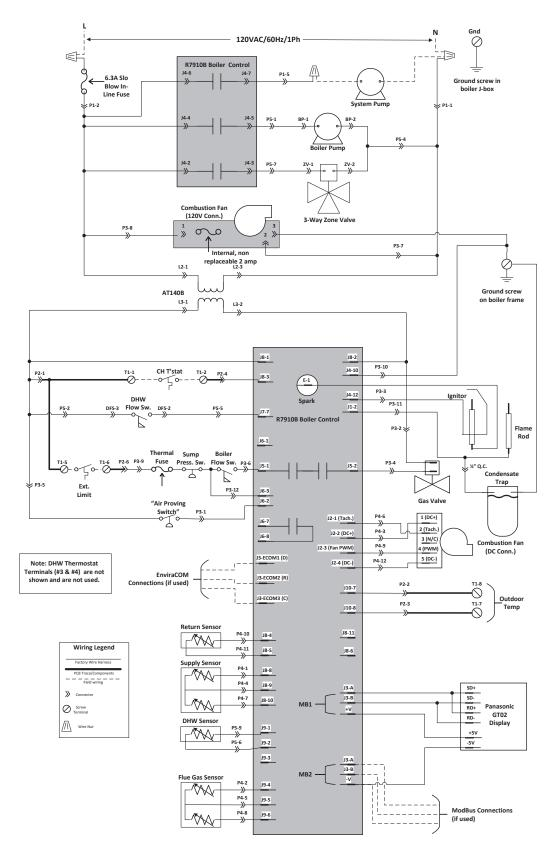
Figure 11.7: Internal Ladder Diagram
