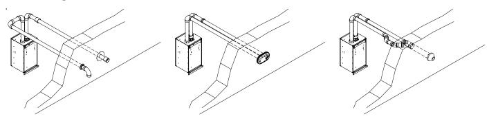
Figure 7.0a: Horizontal Twin Pipe
