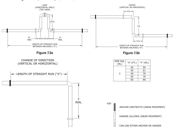
Figure 7.3: Expansion Loops for CPVC/PVC Pipe
