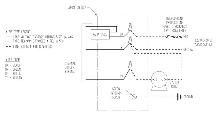
Figure 11.2: Line Voltage Field Connections
