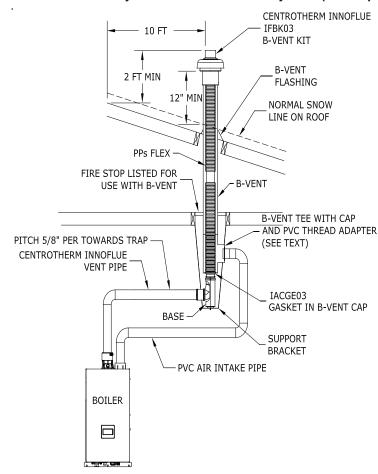
Figure 7.20: Centrotherm InnoFlue B-Vent Air Chase System (Vent Option #10)
