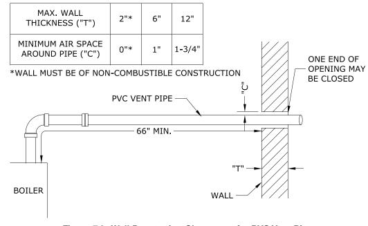
Figure 7.4: Wall Penetration Clearances for PVC Vent Pipe
