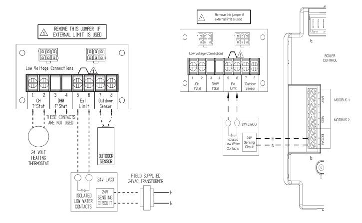
Figure 11.4b: 24 Volt LWCO Field Wiring Using 24 VAC Transformer
