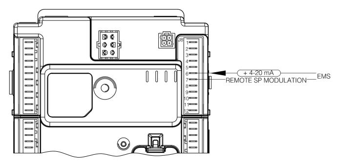
Figure 11.5: 4-20 mA EMS Field Wiring
