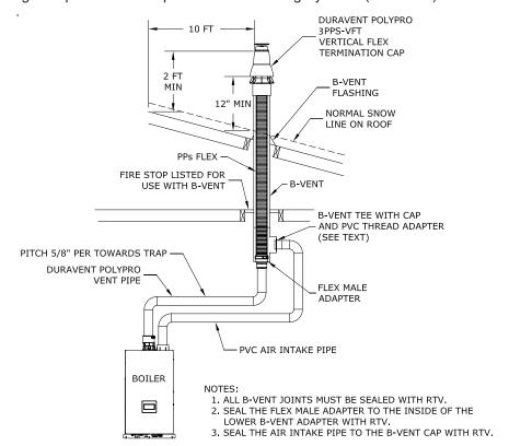
Figure 7.19: Duravent PolyPro B-Vent Air Chase System (Vent Option #9)
