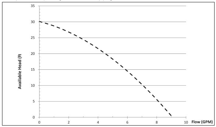
Figure 9.7a: 135 Net Circulator Performance Curve (Taco 0011)
