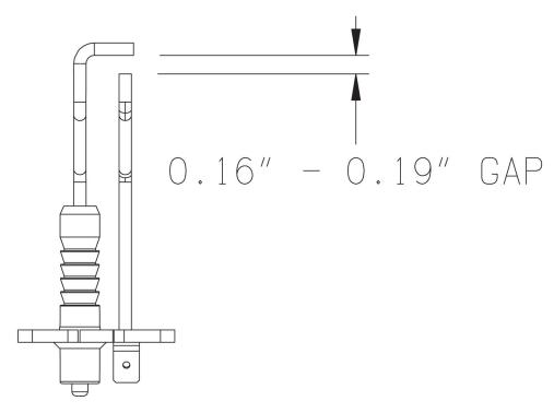
Figure 14.2: Ignition Electrode Gap
