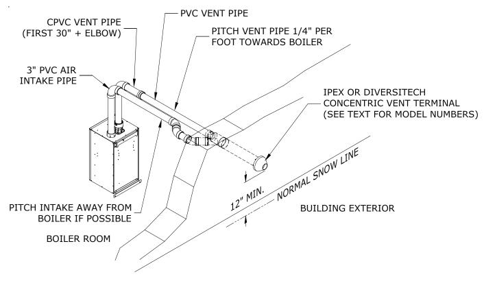
Figure 7.8: Horizontal CPVC/PVC Venting with Concentric Vent Terminal, (Vent Option #1, Terminal Options D & E)
