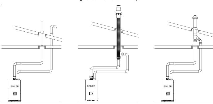
Figure 7.0b: Vertical Twin Pipe
