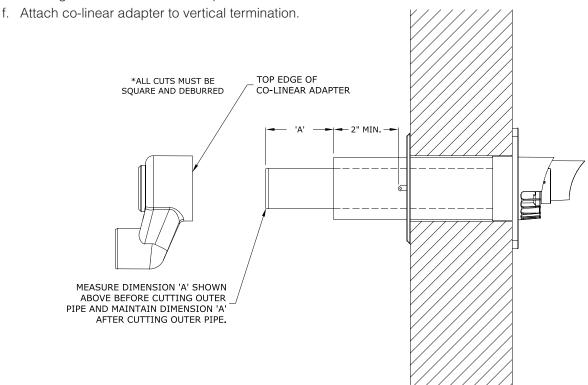
Figure 7.38: Cutting Duravent PolyPro Horizontal Concentric Vent Terminal
