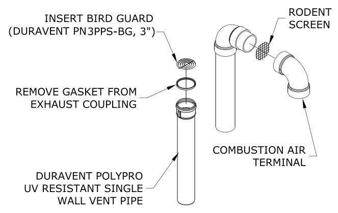
Figure 7.37: Installation of Duravent PolyPro UV Resistant Single Wall Vertical Terminal
