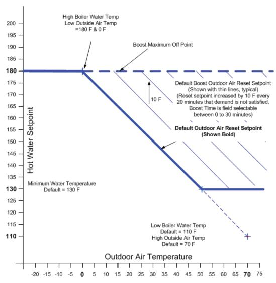
Figure 13.13: Outdoor Reset Curve
