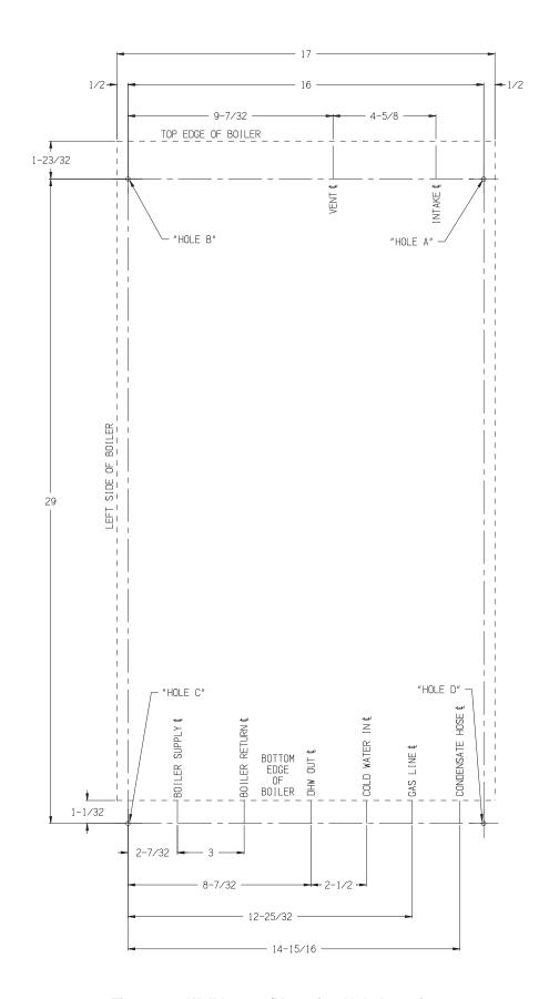
Figure 5.1 Wall Layout/Mounting Hole Location
