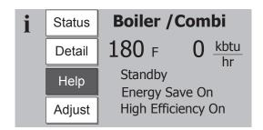
Figure 12.2c: Home Screen with Active Fault
