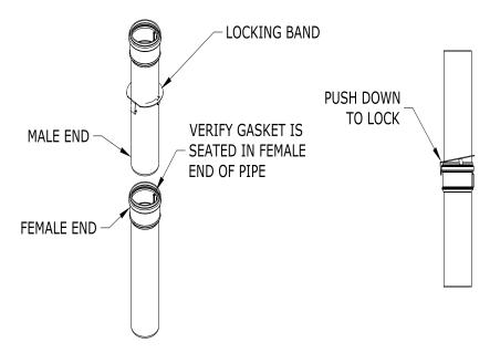
Figure 7.35: PolyPro Locking Band Installation
