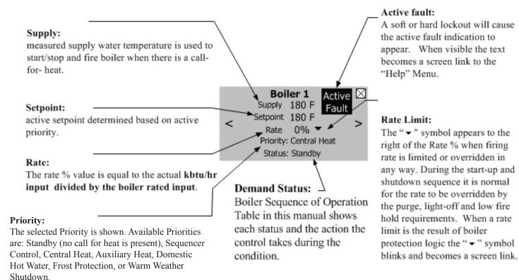
Figure 13.7: Boiler Status Screen Definitions
