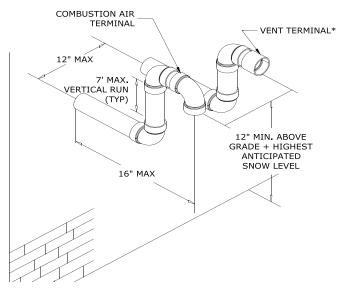
Figure 7.12: Snorkel Terminal Configuration (CPVC/PVC Vent Systems Only)
