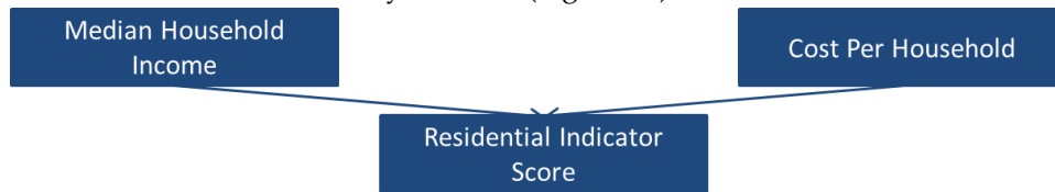
Figure H-4. Divide the CPH by the MHI to determine the RIS.
