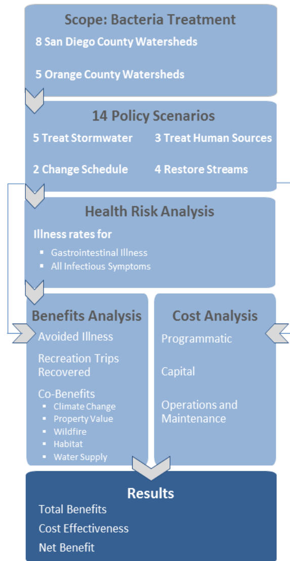
Figure 1: This effort analyzes more than a dozen scenarios to compare their cost effectiveness and net benefit across more than a dozen San Diego and Orange County watersheds.
