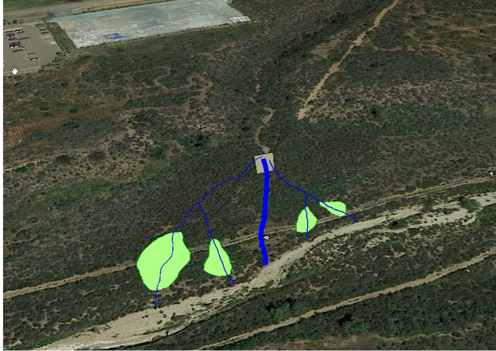
Figure 8 Schematic of Off-line Tributary Wetland: Low flows are diverted by hydraulic structure (tan box) into distributary channels and onto wetlands (green)
