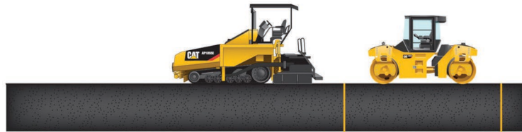
The initial phase roller works close to the paver.
