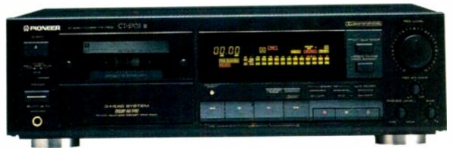
Pioneer's CT-S705 cassette deck utilizes three separate record-and-play heads and features Dolby B and Dolby C noise reduction and Dolby HX Pro; winding time for a 60-minute tape is 100 seconds. Price: $480.
