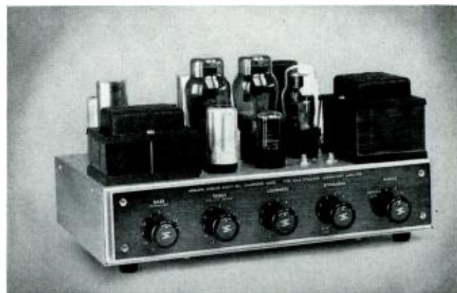
Fig. 3. Single-chassis amplifier with built-in noise suppressor.
