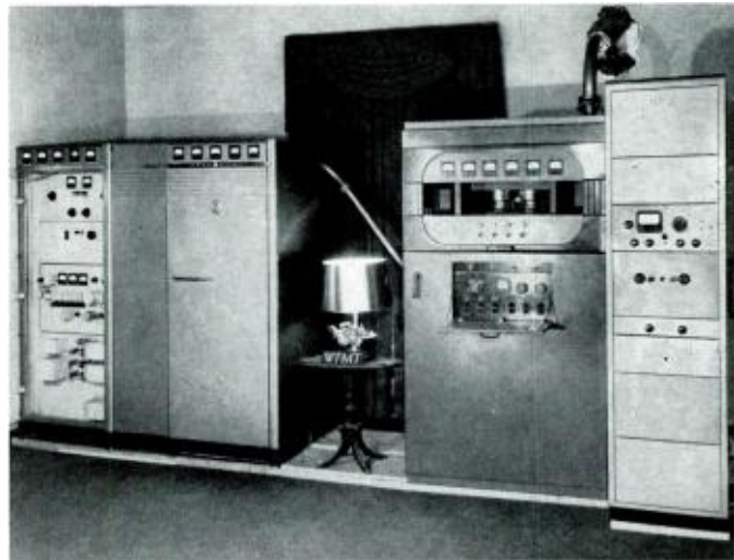
Transmitter room at WFMT. The station has an effective radiating power of 34,000 watts. Equipment here is mostly General Electric.
