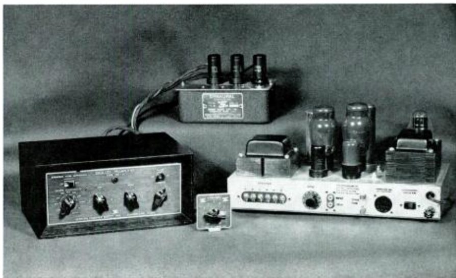
Fig. 1. The complete amplifier system: preamplifier equalizer at left, noise suppressor at center, and power amplifier at right.
