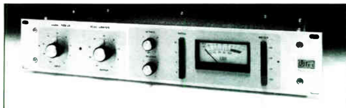
The UREI 1176 LN is a single channel peak limiter with adjustable input, output, attack and release times, compression ratios and meter switching. Stereo coupling is also possible and the unit is available in a two channel configuration, Model 1178.
