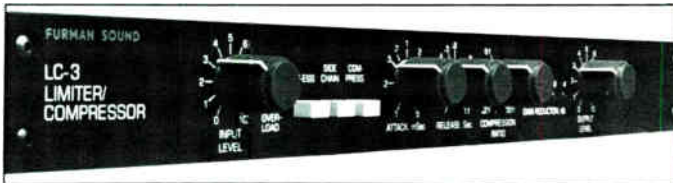
The Furman Sound LC-3 is a single channel compressor/limiter. Features include de-ess and side chain functions, as well as attack, release and compression ratio controls. A stereo link jack is provided, and balanced and unbalanced inputs/outputs are standard.
