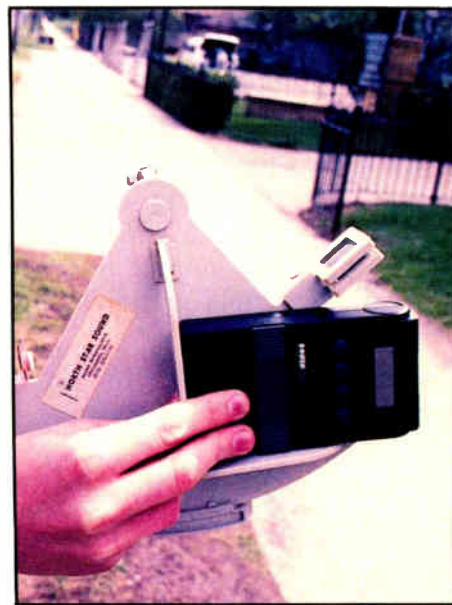
Combination square head rigged to measure distance.
