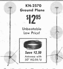
Omnidirectional. Clover leaf top hat for low noise. Beta match puts entire antenna at DC ground. 9' radiator; 9' radiatos, 52-ohms. 5 db circuit gain. 1.5:1 VSWR. Seamless aluminum. With mtg. hardware. Requires 114-156' mast. 4 lbs. Express.
