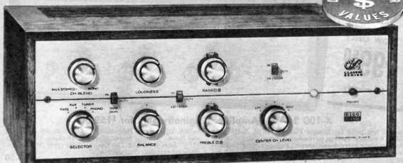
80-Watt Stereo Phono System with Eico 2080K Amplifler Kit
