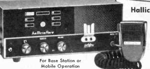
Hallicrafters Model CB-7 6-Channel 5-Watt **CB** Transceiver
