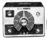
© Model KG-670 Resistor-Capacitor Tester Kit
