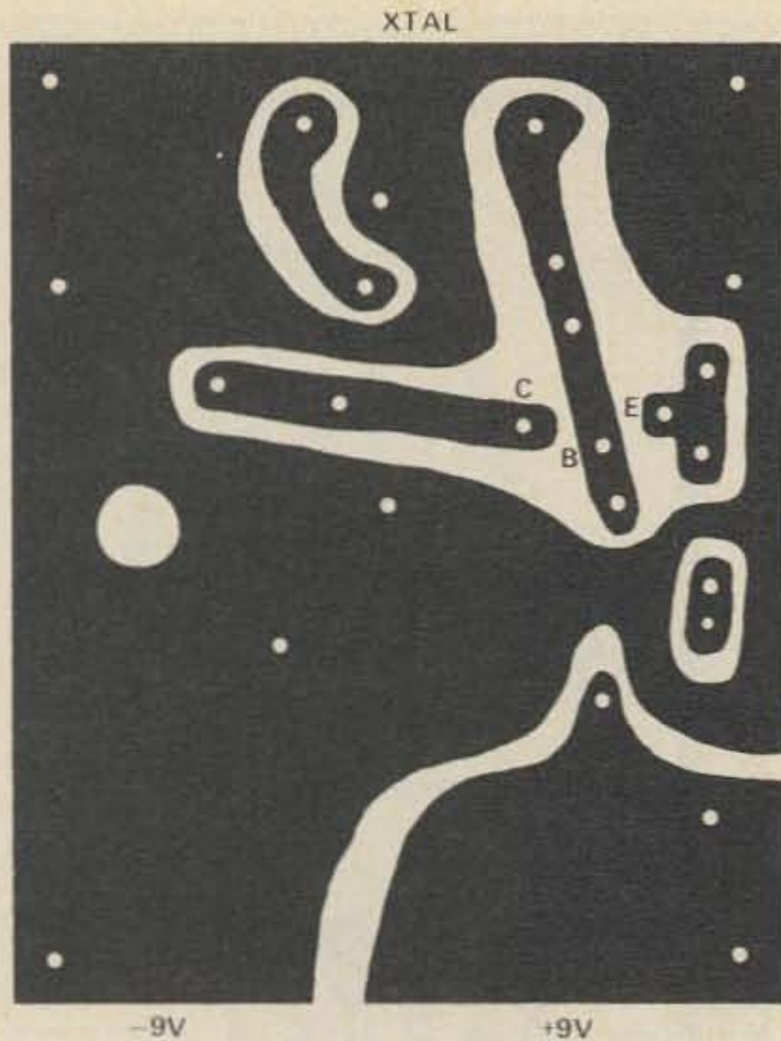
Fig. 2b. Full size layout of crystal oscillator P.C. board.
