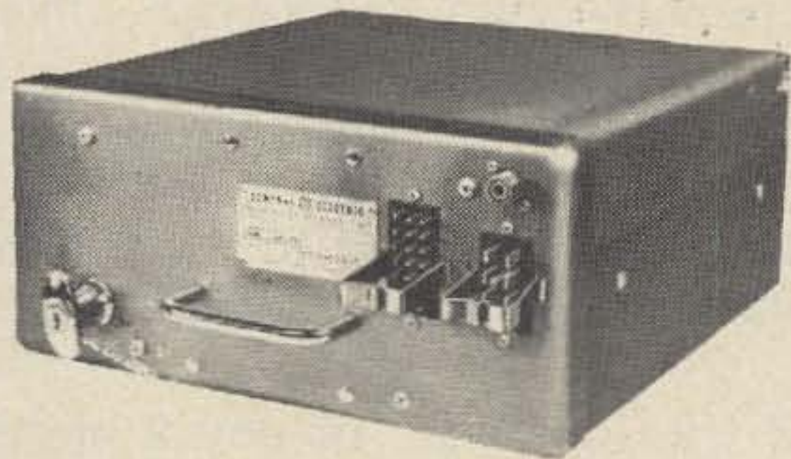
MA/E42 6/12 volts, 15 watts, vibrator power supply
