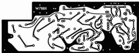
fig. 5. Full-size printed circuit board for the 7-MHz transceiver. Component layout is shown in fig. 4.
