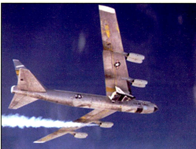
A NASA B-52B carries NASA X-38 experimental test vehicle to drop altitude. (NASA Image)
