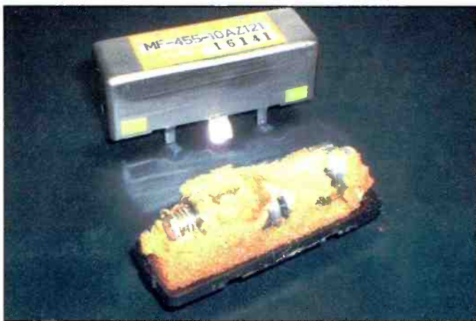
Photo 3: Opening the SSB filter reveals a gooey mass of decaying yellow foam adhering to the mechanical filter's transducers and resonator disks. The weight of the filter had compressed the gooey foam into an almost "superglue"-like substance where the filter components rested on the Bakelite base, destroying the filter's performance.
