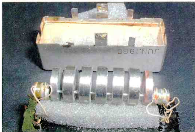
Photo 6: Replacement foam is trimmed to fit and placed between the filter elements and the mounting base, and inside the cover. When assembled, the filter is again gently cradled in soft foam rubber.
