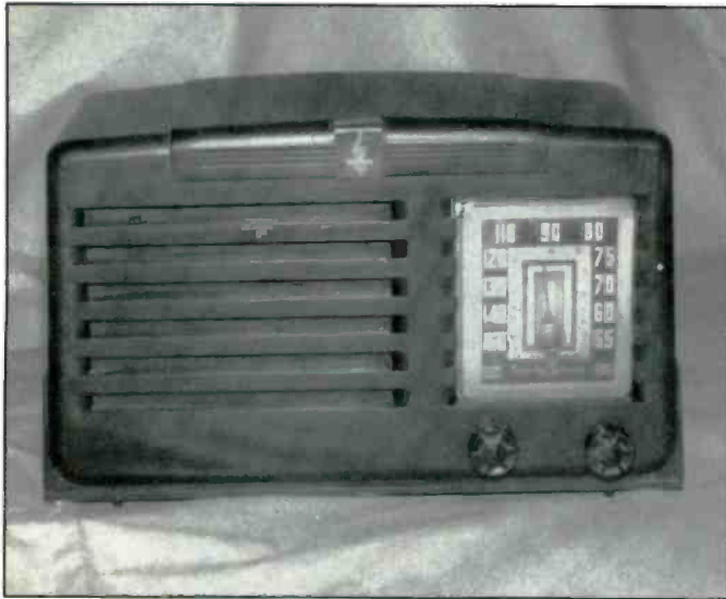
Photo 4. Emerson six-tube bakelite radio, probably dating from the early 1940s. The model number is missing. This radio illustrates a typical AC/DC radio from that era.
