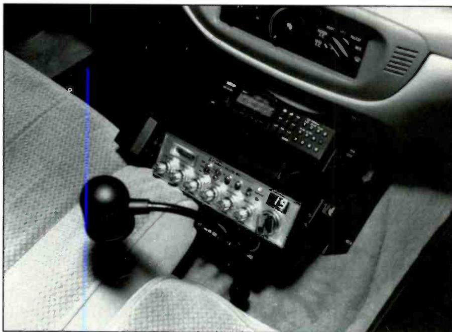
This neat mobile CB—a Cobra 29LTD WX Classic—is a fine rig, but AM-only. Cobra and others have SSB rigs, but they all have the AM mode too.
