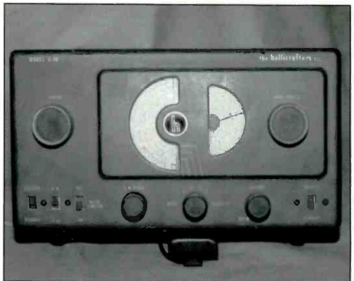
Photo 5. The Hallicrafters S-38 general coverage receiver covered from the AM broadcast band through 30 MHz in four tuning ranges. This early model featured a BFO (Beat Frequency Oscillator) for CW reception, and ANL (AntiNoise Limiting) for improved AM reception.
