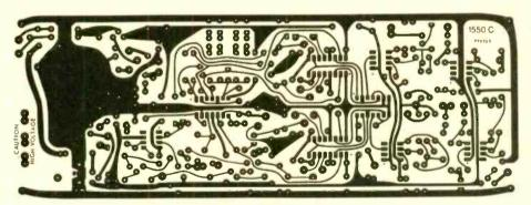
FIG. 14—HALF-SIZE FOIL PATTERNS for the 1550C board. Power supply components are on the extreme left edge. Mixing and chorusing circuits occupy the balance of the board.
