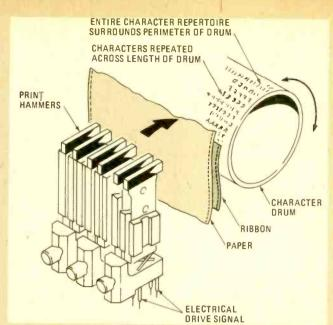
FIG. 2—THE BASIC DRUM IMPACT LINE PRINTER compares the contents of a buffer containing the data to be printed with the position of the desired characters in each print column. At the proper time, the appropriate hammers are activated and the line is printed.
