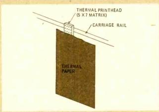
FIG. 6—THE PRINTHEAD OF A THERMAL PRINTER may contain 35 resistive heating elements.
