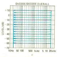
FIG. 7—THE TELEFUNKEN NOISE-REDUCTION compression, expansion and encode/decode curves—a, b and c, respectively.
