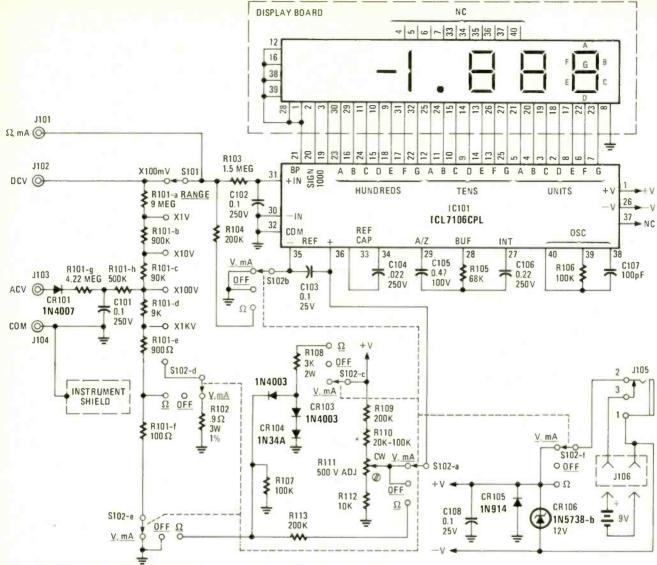
FIG. 1—A COMPACT DMM, the Hickok LX303, based on the Intersil ICL7106 and 3½-digit LCD display. It features auto-zero, auto-polarity selection and automatic over-range indication.
