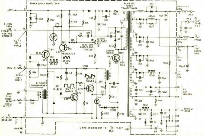
transistor conduct too heavily (thus raising the voltage), the emitter voltage rises, the SCR fires and shunts the drive. The switch is turned off; because an SCR stays on until its anode voltage is cut off, the set must be turned off to reset the SCR.
