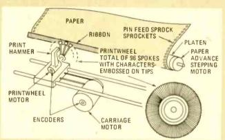
FIG. 3.—A TYPICAL DAISY-WHEEL PRINTER. Many printers use a microprocessor to control the printwheel and the print hammer's Impact force.
