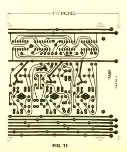
on the 1550A and 1550B PC boards. The 1550A board has some additional circuitry on each end and so is a little longer than the 1550B board. Figures 7 and 8 show the foil patterns for the circuitry at the right and left ends and for the G and C tone blocks. The foil pattern in Fig. 9 is
