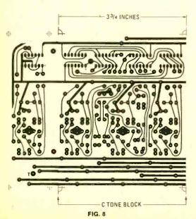
HALF-SIZE SECTIONAL FOIL PATTERNS. Figs. 7 and 8 are right and left ends, respectively, of the "A" board. Fig. 9 pattern is used when making the four tone blocks in the center of boards "A" and "B". Fig. 10 is the F# block and Fig. 11 the C# block on the "B" board.
