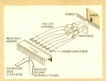
FIG. 5—IN A TYPICAL SERIAL DOT-MATRIX PRINTER MECHANISM like this one from Centronics, a ROM contains the character codes that command the printhead's seven print wires. The ROM's output, fed through power amplifiers, activates solenoids that cause the print wires to impact ribbon and paper.
