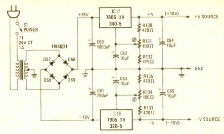
FIG. 5-POWER SUPPLY for the synthesizer uses center-tapped transformer and a full-wave bridge rectifier to deliver equal positive and negative voltages.
