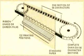
FIG. 4—BAND OR CHAIN PRINTERS are among the fastest units available.
