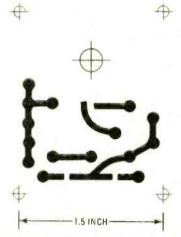
FIG. 16-FOIL PATTERN for the LED board that mounts on the shaft of potentiometer R58.
