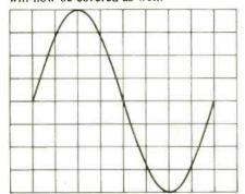
FIG. 8—SINE FUNCTION can be plotted on the CRT screen and used to adjust the sweep generator for minimum distortion.
