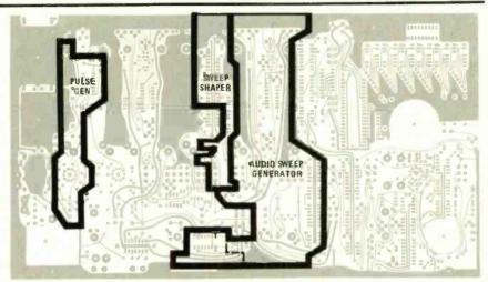
CIRCUIT LOCATION of the pulse generator, sweep shaper and audio sweep generator with respect to the entire PC board.
