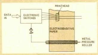
FIG. 7—AN ELECTROSENSITIVE PRINTHEAD creates a spark between the head and the paper. Metal roller completes circuit by contacting paper surface across its full width.
