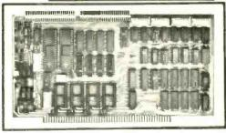
The SwitchBoard™ interface provides 4 parallel ports and 2 RS232/TTY serial ports. Plus strobe and attention ports. Plus, onboard facilities for 4K of optional static RAM and 4K of user-supplied EPROM (sockets provided).
