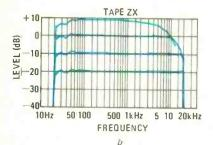
FIG. 5—FREQUENCY RESPONSE of Nakamichi's type SX treated-ferric tape (shown in a) and their prototype ZX metal-alloy tape (shown in b).
