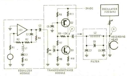
FIG. 4—SIMPLIFIED SCHEMATIC of the Actilinear recording circuit.
