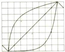
FIG. 9—CALIBRATION WAVEFORMS. Log function is shown in  $\boldsymbol{a}$ , triangular wave is shown in  $\boldsymbol{b}$  and antilog function is shown in  $\boldsymbol{c}$ .
