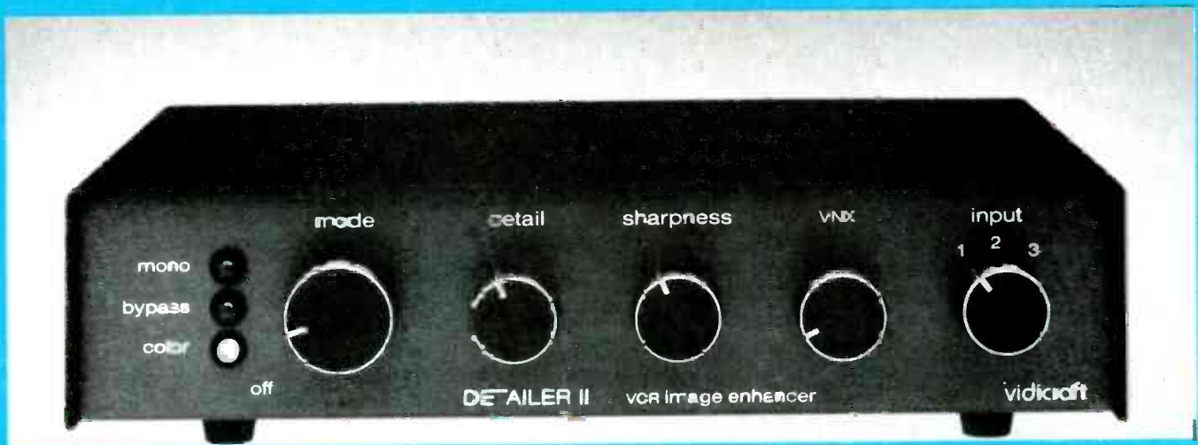
THE SHARPNESS AND DETAIL of both recorded and broadcast video can be improved by using an image enhancer.
