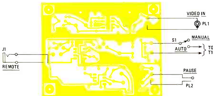
FIG. 6—OFF-THE-BOARD connections. Use RG-174 coax for VIDEO IN cable.
