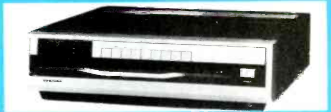
AMONG THE FEATURES of this VP-500 CED videodisc player are stereo audio and CX noise reduction.
