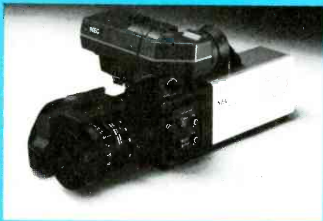
SOLID-STATE IMAGE SENSORS, such as the one used in this NEC TC-100 color camera may eventually replace the cumbersome and power-hungry image tubes of today.
