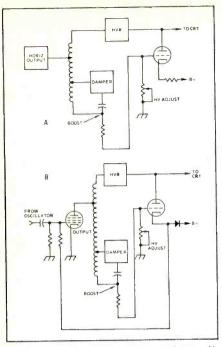
Fig. 6—Shunt-type high-voltage regulators. A) Without holddown provision. B) With holddown provision.
