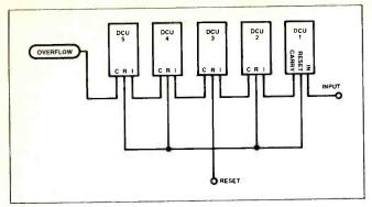
Fig. 1—A decimal counting assembly (DCA) consists of several decimal counting units (DCU's) in cascade. Each DCU counts from 0 to 9 and controls one digit of the multi-digit display.
