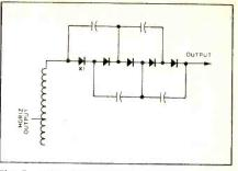
Fig. 5-Solid-state high-voltage supply.
