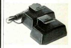
the antenna where they are strongest and free from interference. The unit provides a gain of 16 dB or over five times the input level.
