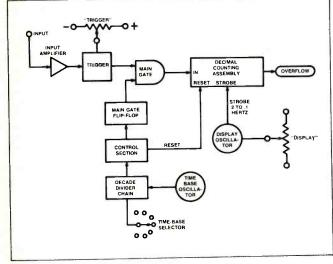
Fig. 3-Block diagram of a typical frequency counter.
