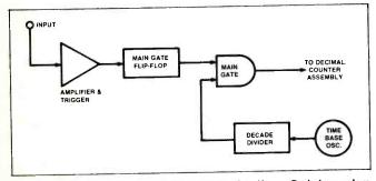
Fig. 4—Block diagram of period counting functions. Period counters measure the time interval between the beginning of successive pulses by reversing the function of the input amplifiers and the time base viz a viz the control flip-flop.
