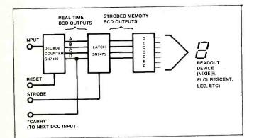
Fig. 2--Simplified block diagram of a low-cost TTL decimal counting unit capable of counting to over 20 MHz. The latch circuit keeps the display stable.
