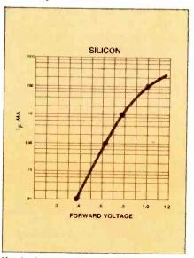
Fig. 1—Forward voltage—forward current curve of a typical silicon bipolar transistor.
