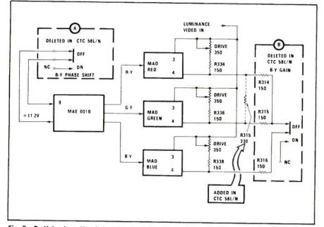
Fig. 8—Partial schematic of the ACM IV circuit used in other XL-100 color TV chassis, with the CTC58 chassis noted. Courtesy of RCA.
