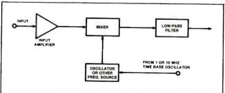
Fig. 9—Heterodyning is another method of extending the frequency range of a digital counter.
