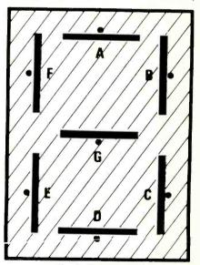
Fig. 3—The simplified illustration shows how the digits zero through nine can be formed by illuminating various sections of the sevensegment display forming channel numbers. Courtesy of RCA.
