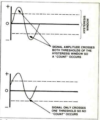
Fig. 5—A "count" can be achieved only when the input signal crosses both the upper and lower bounds of the trigger's hysteresis window.
