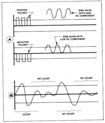
Fig. 7—Several of the waveforms which cannot be counted by a digital counter with a fixed hysteresis window.
