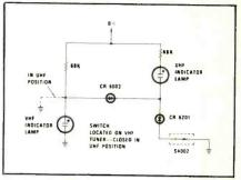
Fig. 7—Simplified schematic diagram showing the separate pair of neon lamps used to indicate VHF or UHF reception. Courtesy of RCA.
