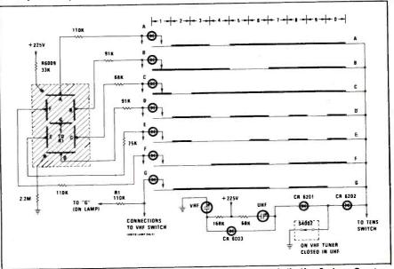
Fig. 5-Simplified illustrations showing the Units section of the UHF Indicating System. Courfesy of RCA.
