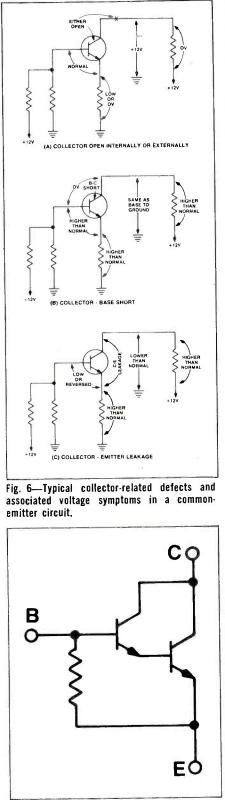
Fig. 7—Internal circuitry of a Darlington transistor.
