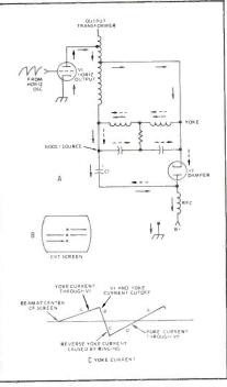
Fig. 1—Horizontal deflection circuit.
