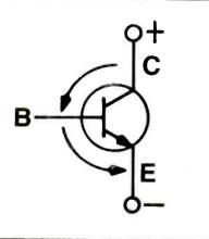
Fig. 3—The leakage current indicated by the arrows is the reason that germanium power transistors inherently have low reverse-bias emitter-to-collector resistance.
