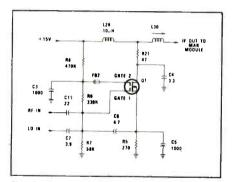
Fig. 1—The two-transistor, "cascode-type" VHF mixer has been replaced with a dual-gate MOSFET mixer. Courtesy of RCA.
