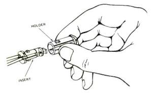
ment as usual, but to separate the holder from the insert the holder must be gripped as shown in illustration and squeezed to unlock it. This new assembly may be used to replace all original holders with the part number 142848 or 143290. ■
