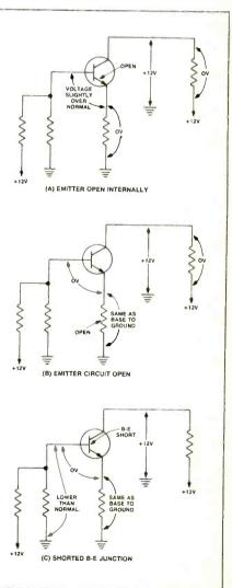
Fig. 4—Typical emitter-related defects and associated voltage symptoms in a commonemitter circuit.
