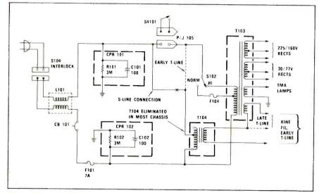
Fig. 2—Schematic diagram showing the changes made in the power supply employed in the CTC68 color TV chassis. Courtesy of RCA.
