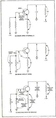
Fig. 5—Typical base-related defects and associated voltage symptoms in a common-emitter circuit.
