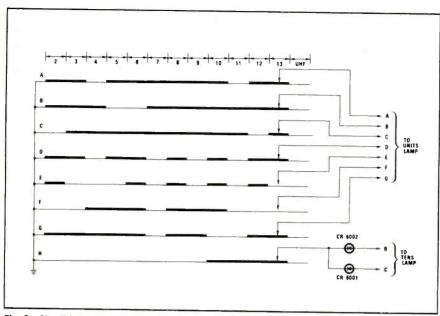
Fig. 6—Simplified schematic diagram showing the VHF Channel Indicating System. It is similar to the units section of the UHF switch. Courtesy of RCA.
