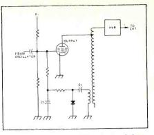
Fig. 8-Diode feedback high-voltage regulator.
