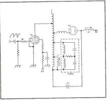
Fig. 2—Horizontal deflection circuit, showing linearity control.
