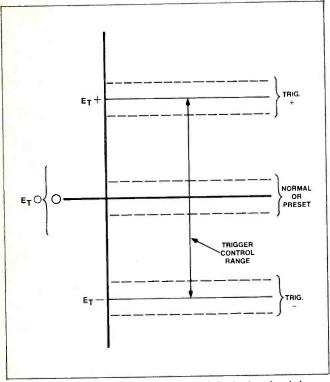
Fig. 6—Trigger controls vary the position of the hysteresis window up and down on a voltage scale so that signals of either polarity, with or without a DC component, can be counted.
