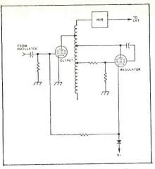
Fig. 7—A pulse-type high voltage regulator.
